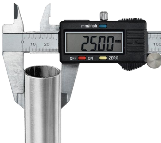
Figure 1 - Measuring the external dimension of the tube with a caliper gauge. Outcome example: 25 mm
