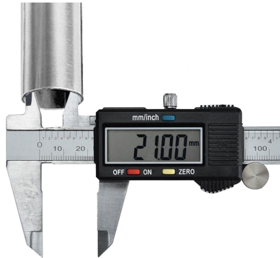
Figure 3 - Measuring the inner tube size with a caliper. In this example, the inside measurement is 21 mm
