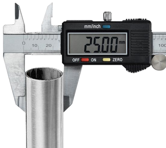
Figure 1 - Measuring the outer tube size with a caliper. Outcome example: 25mm
