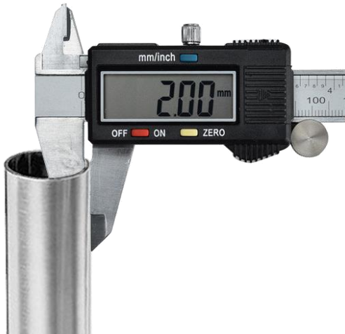
Figure 2 - Measuring the wall thickness with a caliper gauge. In this example, the wall thickness is 2 mm
